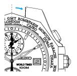
If daylight saving time is used in a city on the bezel, an arrow mark is printed to the right of the city marker.
